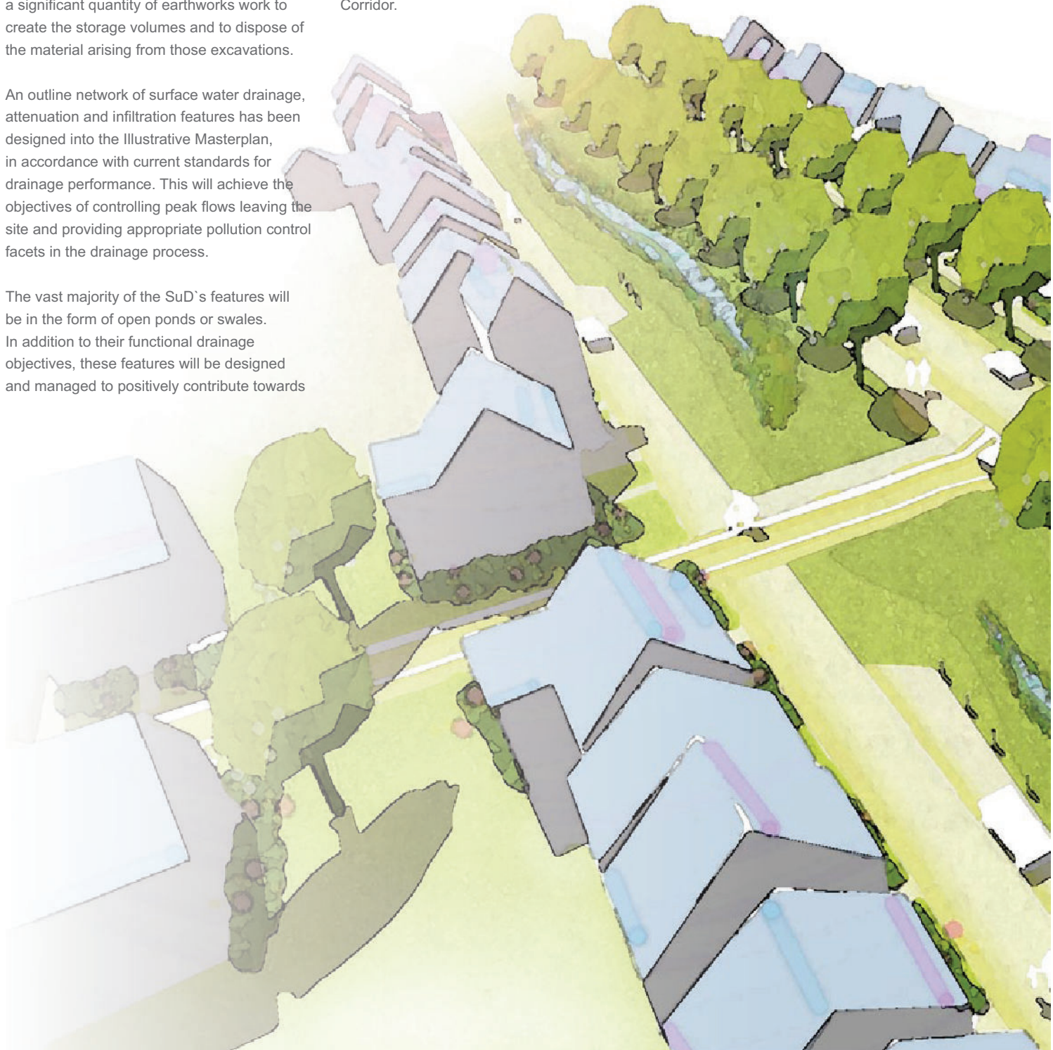
Indicative sketches showing how SuDS swales and linear ponds could be incorporated into the design of the streets and GI corridors
